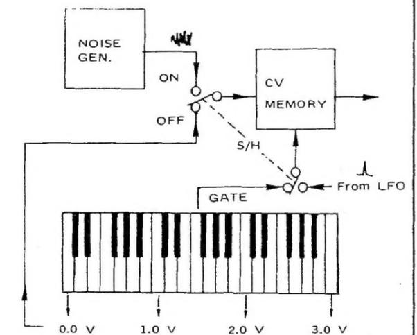
The voltage on S1A pin 2 charges up the memory capacitor (C13) through Q5. Q5 is turned on by the Gate generator or the LFO trigger pulse through CR4. Q6 and Z1A are an FET op amp follower with high input impedance to buffer the voltage on C13. The output of the Keyboard Control Voltage Memory circuit is supplied to the control inputs of the VCO and the VCF via J4-1 and J4-3.
